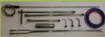
Stack Monitoring Kit VBSS1 can be used to measure total emission of Particulate Matter and Gaseous Pollutants from all types of industries including Thermal power stations, Steel Plants, Chemical Plants and Cement Industry. It can be used to take accurate representative samples of Particulate Matter and various Gaseous Pollutants like SO2, NOx, etc from the stack in accordance with the methodologies developed by USEPA and as specified by Central Pollution Control Board in Emission Regulation.
